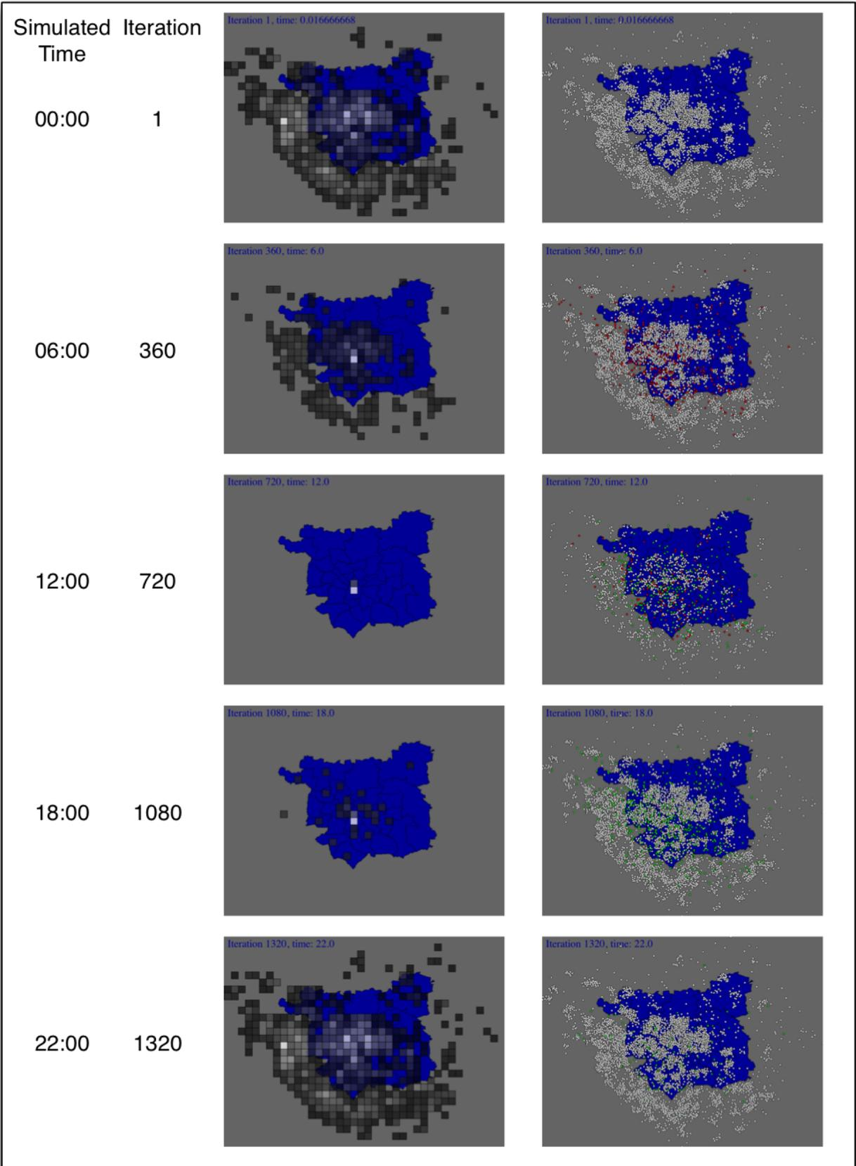
**Fig. 2.** The prototype model running over a single simulated day (uncalibrated). Agents travel from within Leeds and the outskirts of the city towards the central business district. The left maps show density (white cells are the most densely populated). On the right maps, white points indicate stationary agents, red signifies agents travelling to work and green shows agents travelling home.
